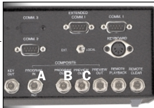
Close-up of PVI-64 ports
